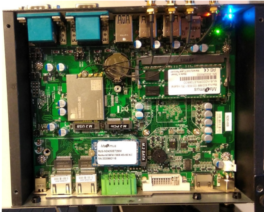
Figure 11: SIMCom SIM8202G-M2 module embedded on a Pico-ITX motherboard
