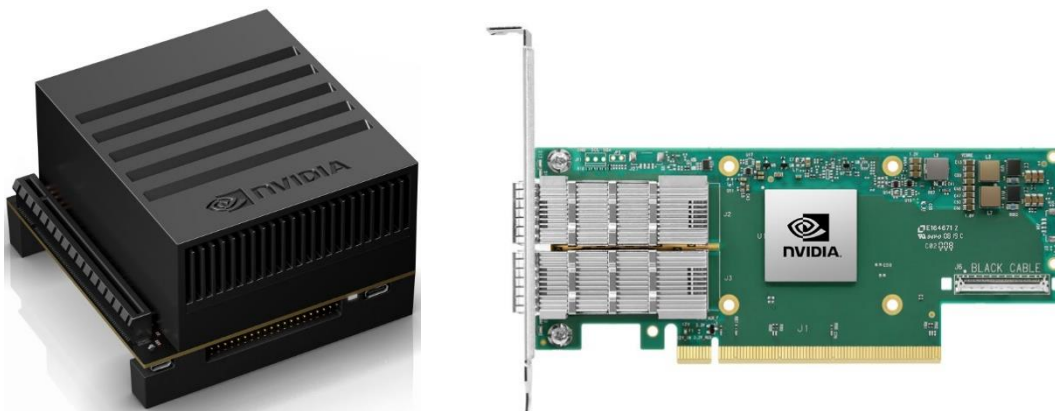
Figure 47: Jetson AGX Xavier Development Kit and ConnectX-6 NIC
