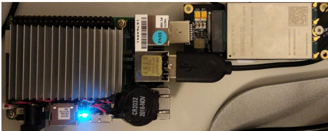
Figure 12: Quectel RM500Q-GL module connected over USB to an "UP Board"
