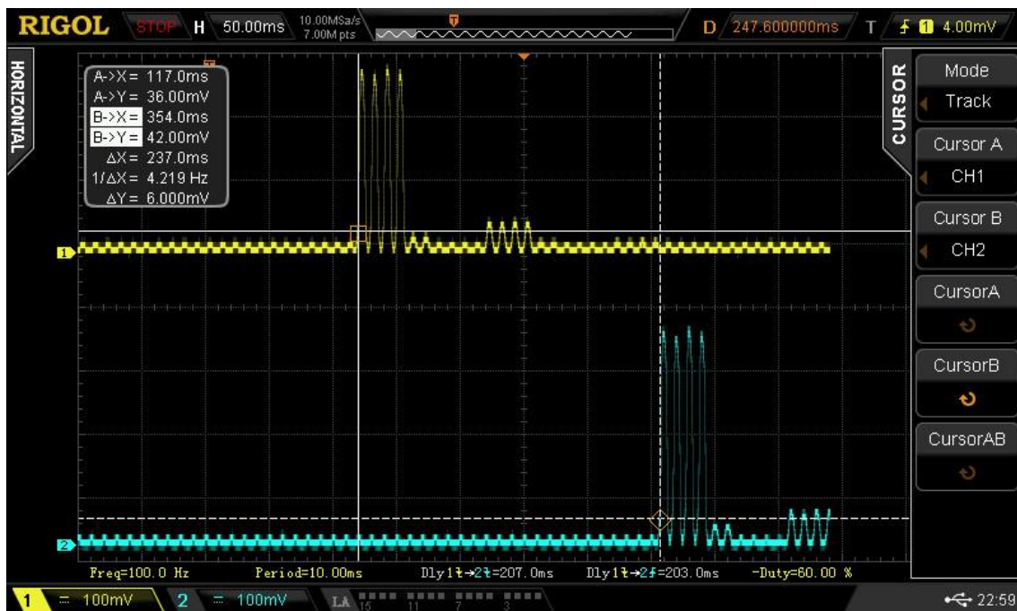
Figure 67. 10Mbps @ 50fps, Latency= 237ms, De-jitter buffer = 200 ms
