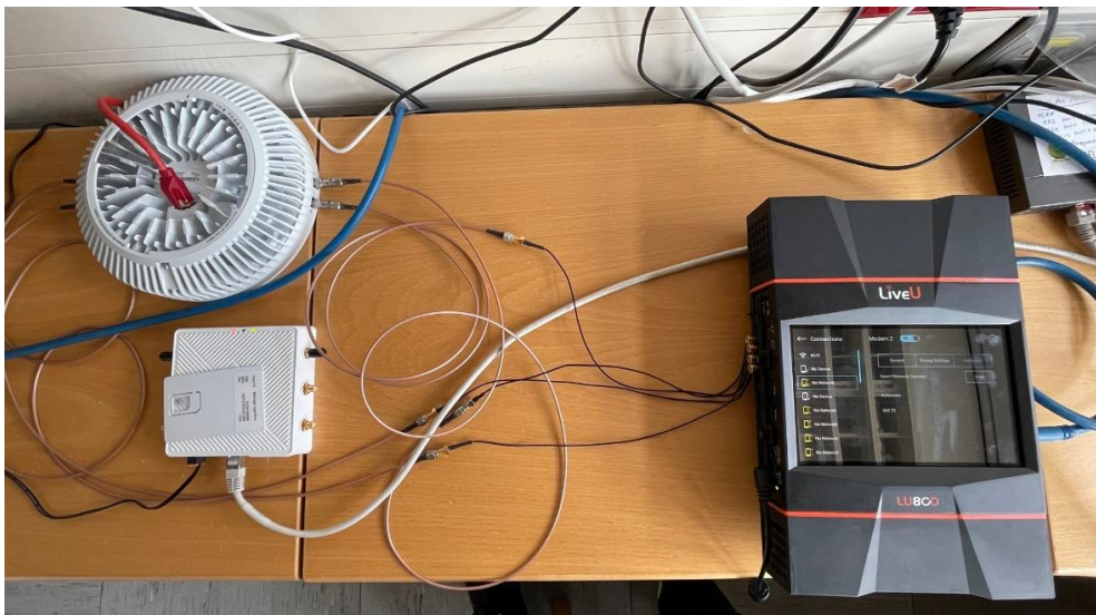
Figure 49 LU800Pro connected to Ericsson 5G lab network via external 5G modem
