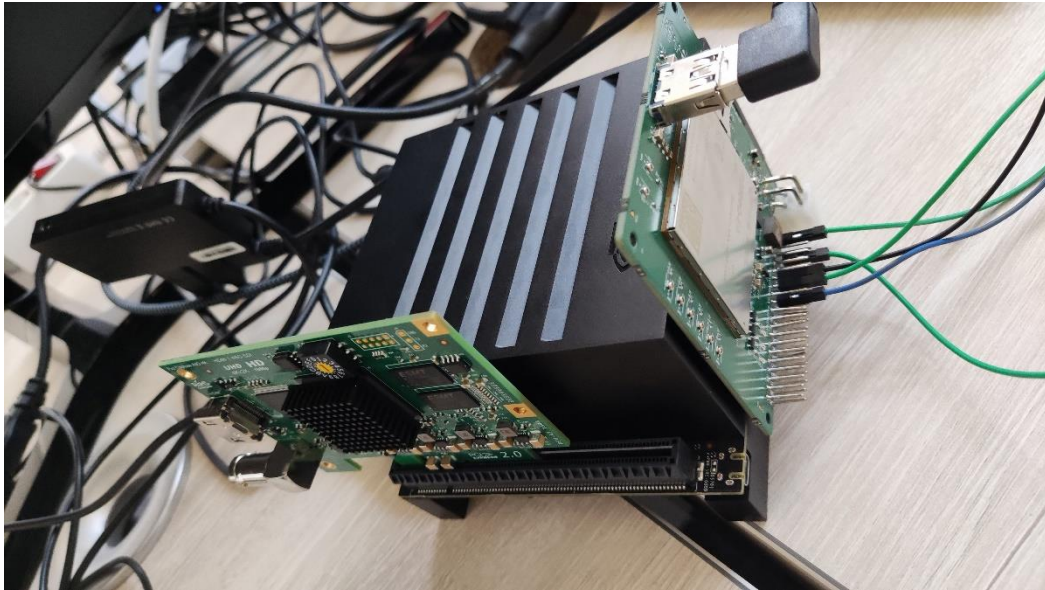
Figure 31. Interconnection of all components in the portable solution, without case
