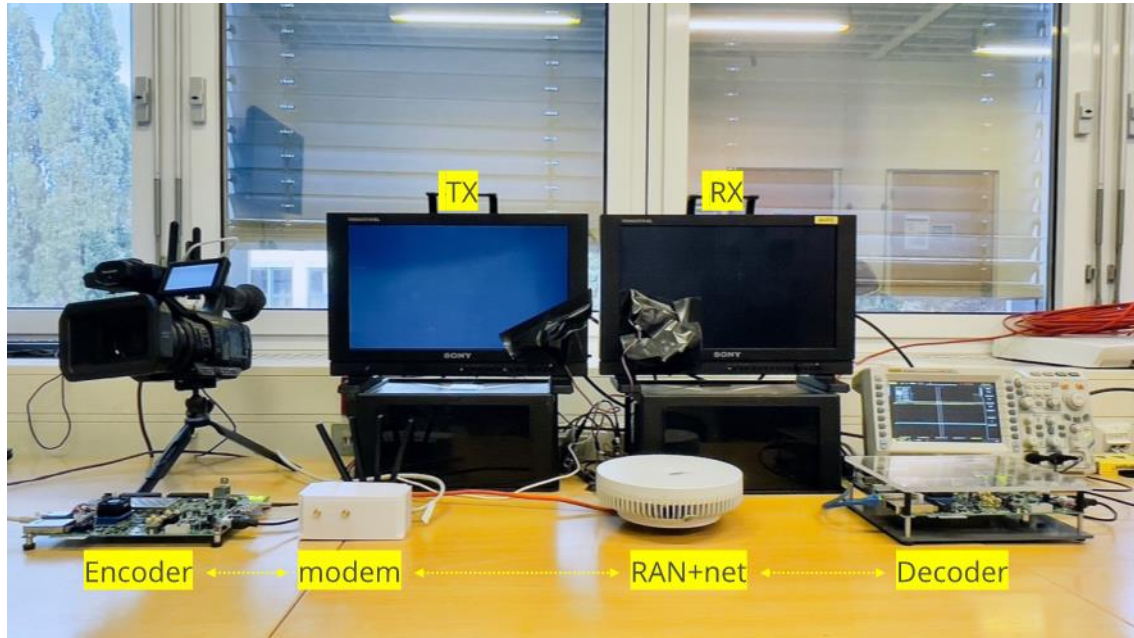
Figure 12 - The setup in the 5G lab
