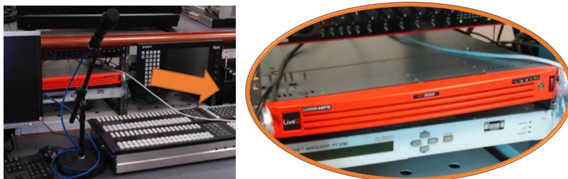
Figure 14 - LiveU LU2000SMPTE HEVC decoder-receiver
