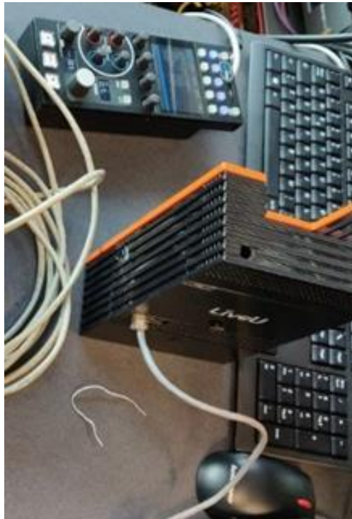
Figure 32 - Cyanview remote camera control via LiveU IP PIPE
