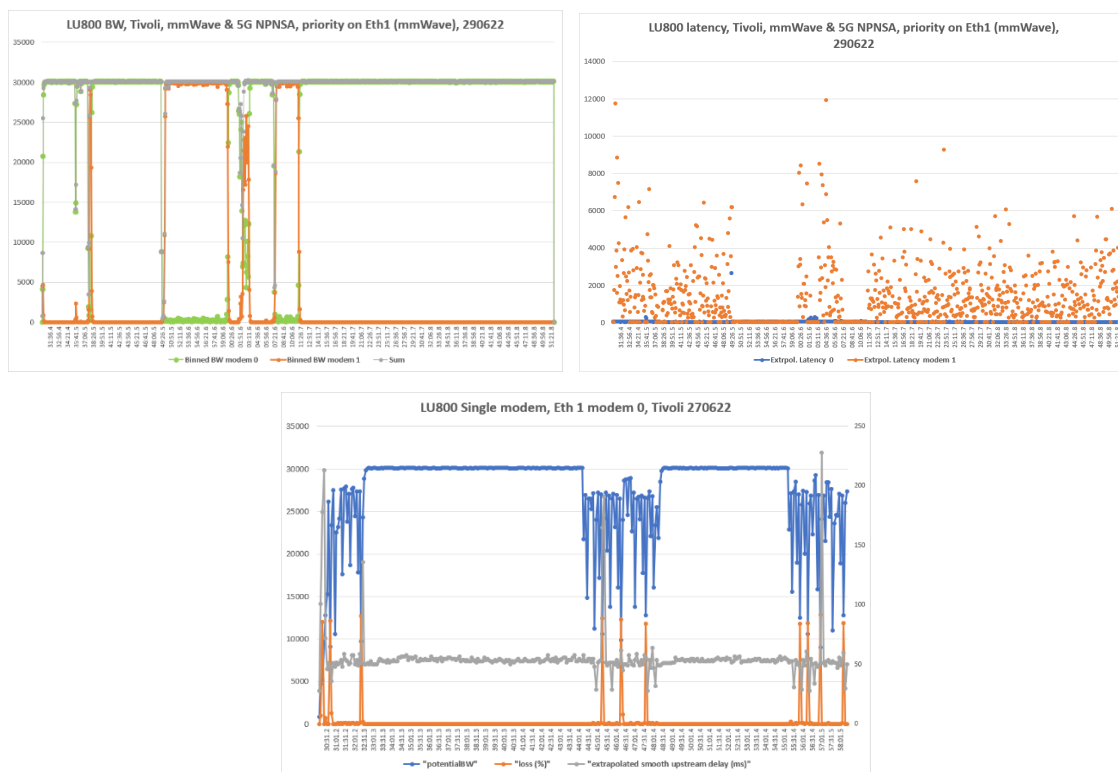
Figure 98: Results for 2 modems bonding, 5G mmWave and SNPN for remote production trial in Tivoli.
