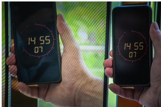
Figure 92: Glass to glass latency, showing 180ms latency during the Tivoli Trial.
